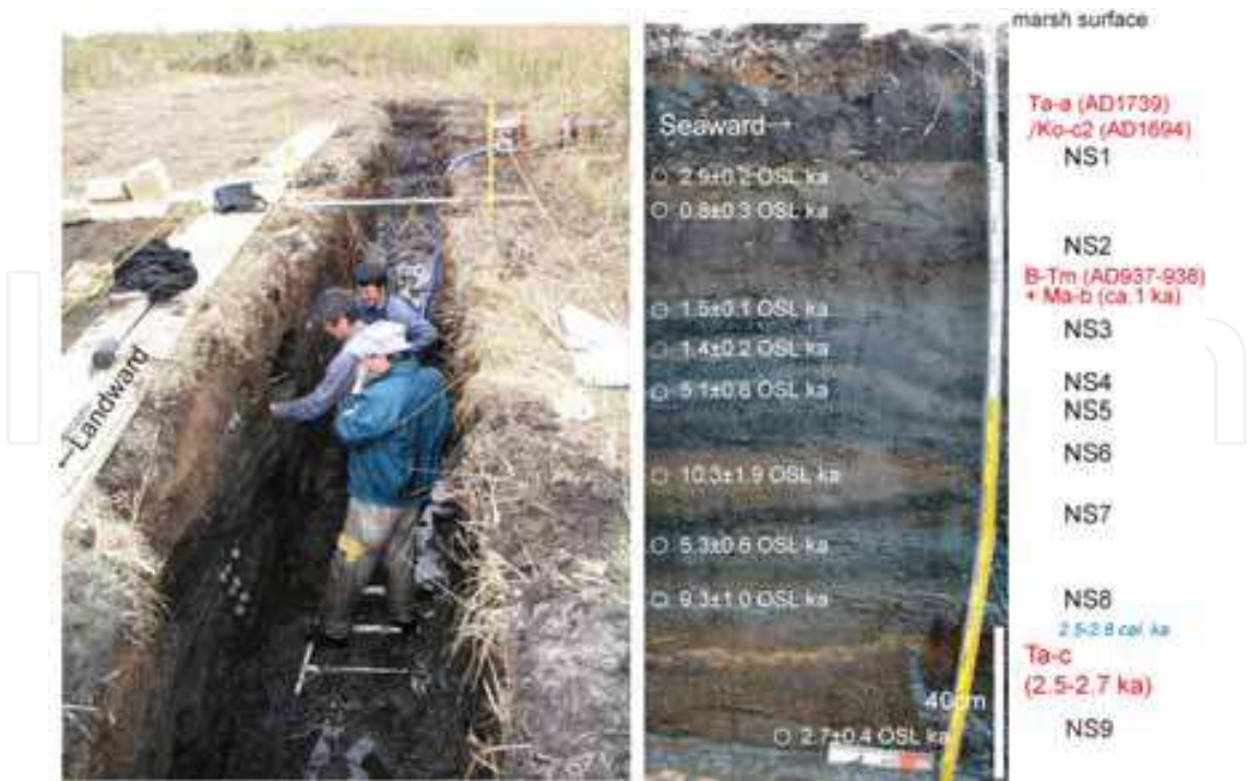
Fig. 6. Collection of samples for OSL dating at Shig trench (left). Photograph of the trench wall showing the OSL sampling horizons and dating results (right). AMS 14 C dating results, tephra layers and dates, and sand beds NS1 to NS9 are indicated to the right of the photograph.
