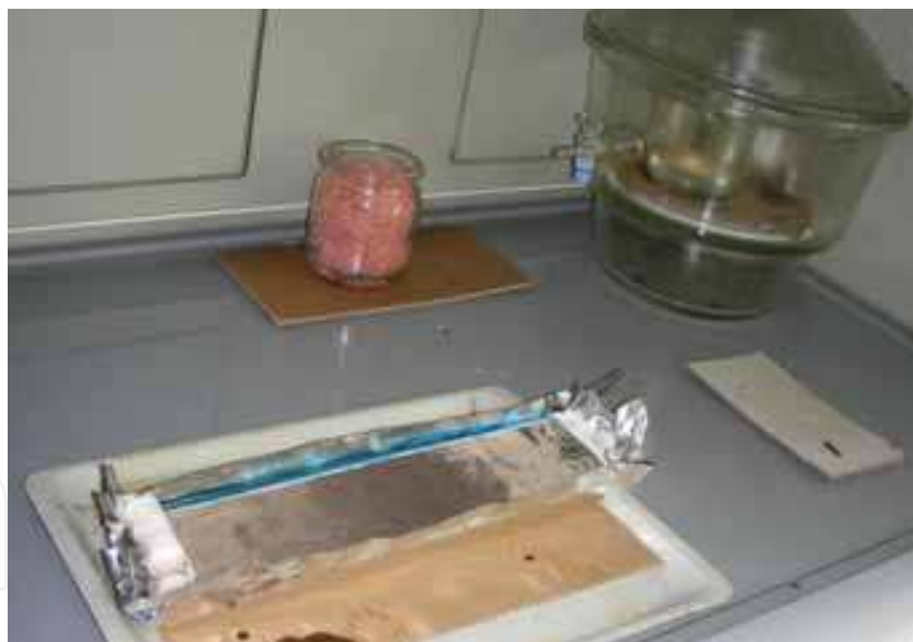
Fig. 6. Impregnation of the soft core sediment to get a hardened sample for the preparation of a thin section (from Srisutam & Wagner, 2010c)
