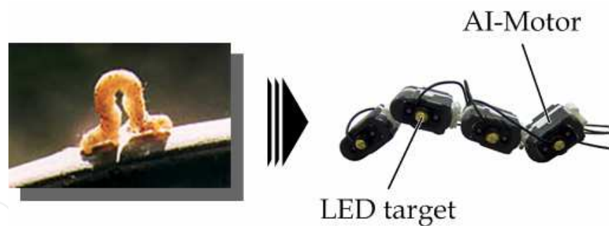
Fig. 1. Caterpillar-shaped robot for Q-learning of advancement motion: only the AI-Motors at both the sides are enabled
