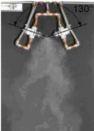
Fig. 4. Spraying technique with jet impact method
