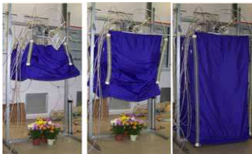
Fig. 24. Example of textile cover sheet retraction/ extension in the laboratory
