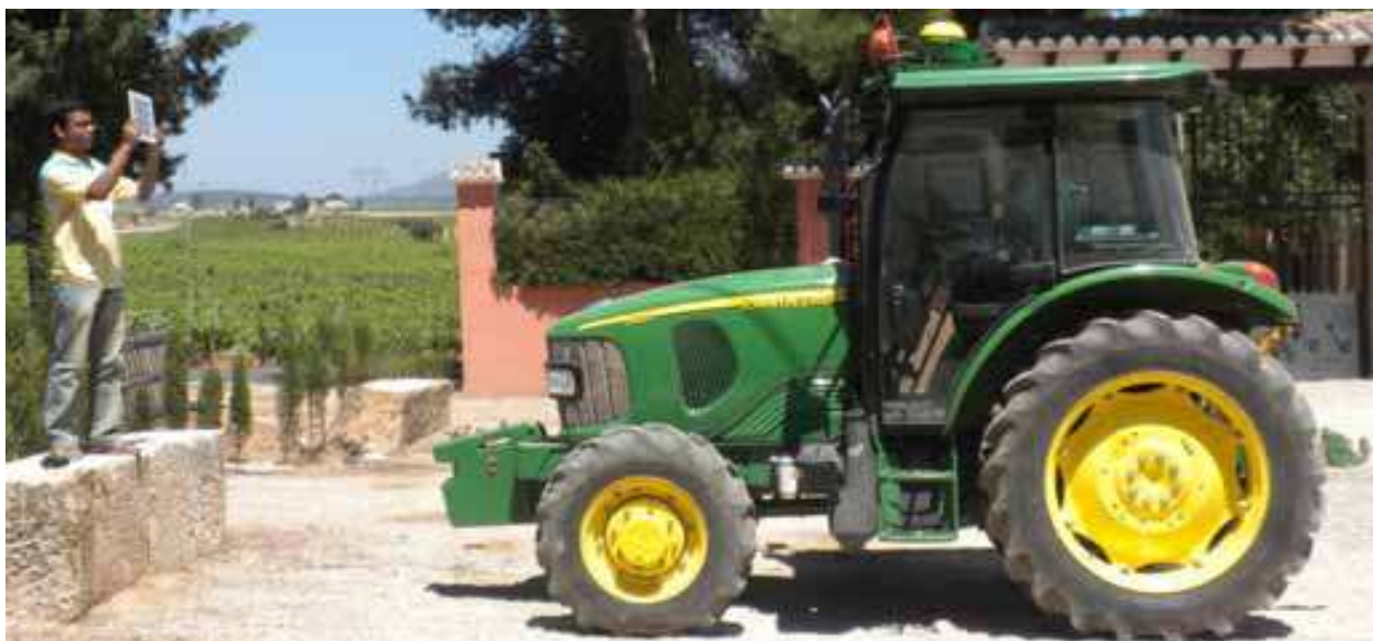
Fig. 1. Calibration procedure for non-precalibrated stereo cameras
