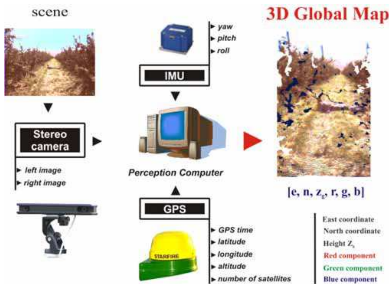
Fig. 7. System architecture for a stereo-based 3D terrain mapping system
