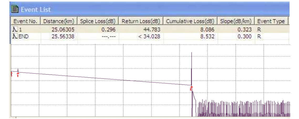
Fig. 36. 1310nm SMF at 200ns pulse width (manually measurement)
