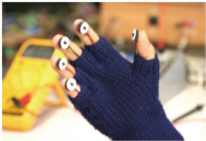
Fig. 5. Tactile sensors bounded on fingers hand
