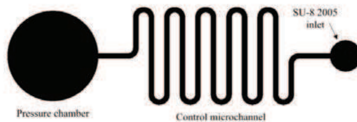
Fig. 11. Layout SU-8 mask for a pressurized chamber.
