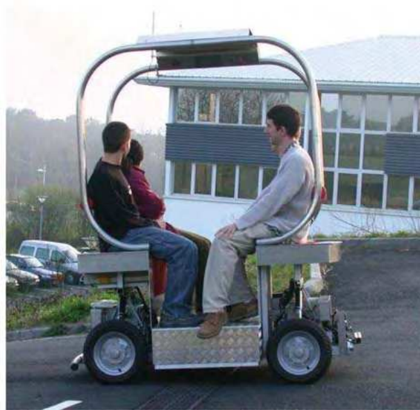
Fig. 9. Robucab mobile robot platform transporting four people.
