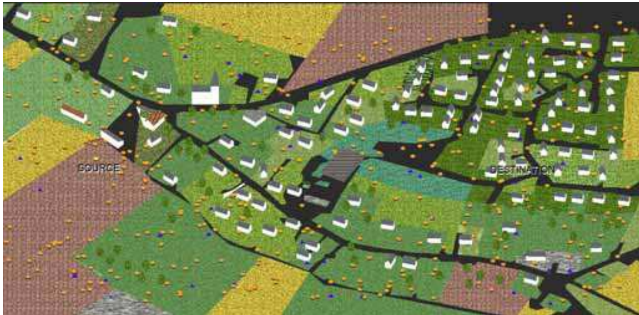
Fig. 11. Test case for LDR representing an obstructed simulated field. Sensors are represented by a circular shape and mobiles with a triangular shape.
