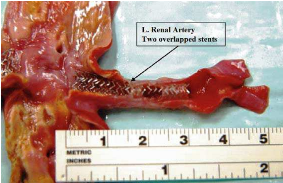
Fig. 8. Partially exposed explanted aortic segment with the left renal artery demonstrating position of the implanted overlapped stents fatigue cycling with a mean stress not equal to zero. It should be noted that mean stress could also be a result of the plastic deformations of crimping and deployment. The Goodman relation states that fatigue failure will occur if the stress state in the component satisfies the relation:
