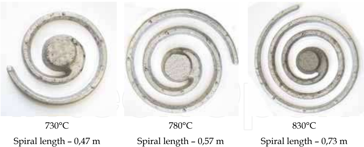
Fig. 4. Spiral casts of Elektron 21 alloy after fluidity test.
