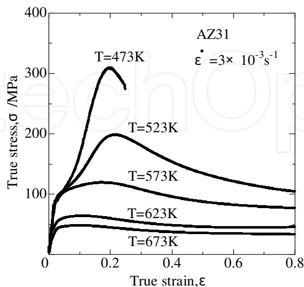
Fig. 3. Temperature effect on true stress-true strain curves of as-annealed AZ31 alloy with a grain size of  $22.3 \mu\text{m}$  during single pass compression at a true strain rate of  $3 \times 10^{-3} \text{ s}^{-1}$ .
