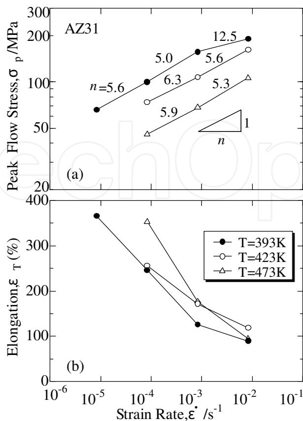
Fig. 19. Strain rate dependence of (a) peak flow stress  $\sigma_p$  and (b) total elongation to fracture  $\varepsilon_T$  of MDFed Mg alloy tested at 393K, 423K and 473K.
