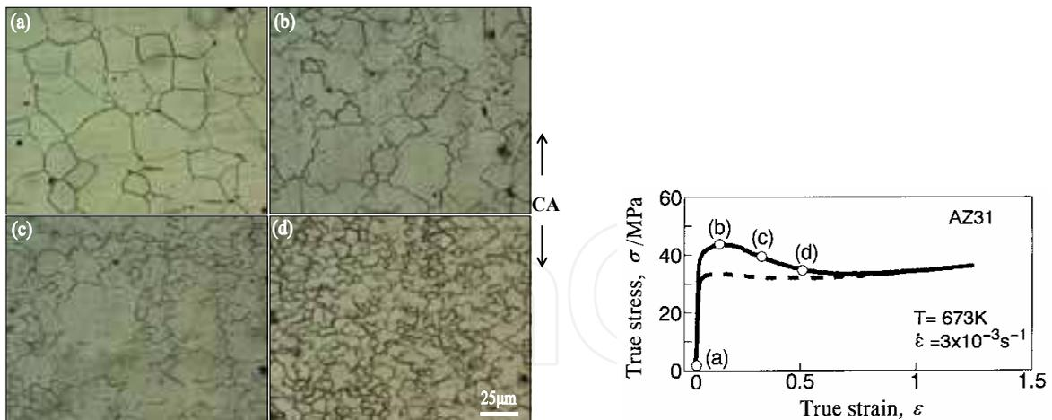
Fig. 4. Typical optical microstructures and the corresponding true stress-true strain curve of AZ31 alloy deformed to various strains at 673 K and at  $3 \times 10^{-3} \text{ s}^{-1}$ , followed by water quenching. The compression axis (CA) was parallel to the extrusion direction of the alloy. (a)  $\varepsilon = 0$ , (b)  $\varepsilon = 0.1$ , (c)  $\varepsilon = 0.3$  and (d)  $\varepsilon = 0.5$ .
