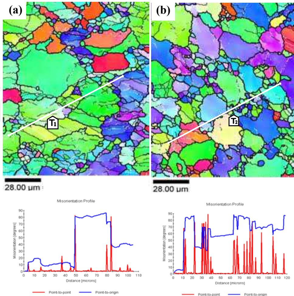
Fig. 10. OIM maps of Mg alloy AZ31 deformed to  $\varepsilon = 0.3$  at 573 K by (a) a single- and (b) two-directional compression with changing the loading direction. Point-to-point misorientations and lattice rotation measured along the lines  $T_1$  and  $T_2$ .
