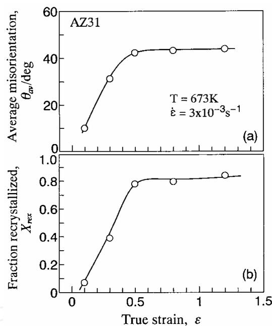
Fig. 6. Strain dependence of (a) average misorientation of (sub)grain boundaries,  $\theta_{av}$ , and (b) fraction dynamically recrystallized,  $X_{rex}$ , of AZ31 alloy deformed at 673 K and at  $3 \times 10^{-3} \text{s}^{-1}$ .
