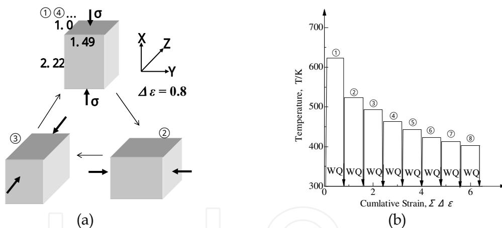
Fig. 1. Schematic illustration of the thermo-mechanical processing used in MDF with continuous decreasing temperature in each pass. (a) The loading direction is changed in  $90^\circ$  with pass to pass ( $x \rightarrow y \rightarrow z \rightarrow x \dots$ ). A pass strain  $\Delta\varepsilon$  is 0.8. (b) Deformation temperature is decreased from 623K to 423K in each MDF. WQ indicates water quenching.
