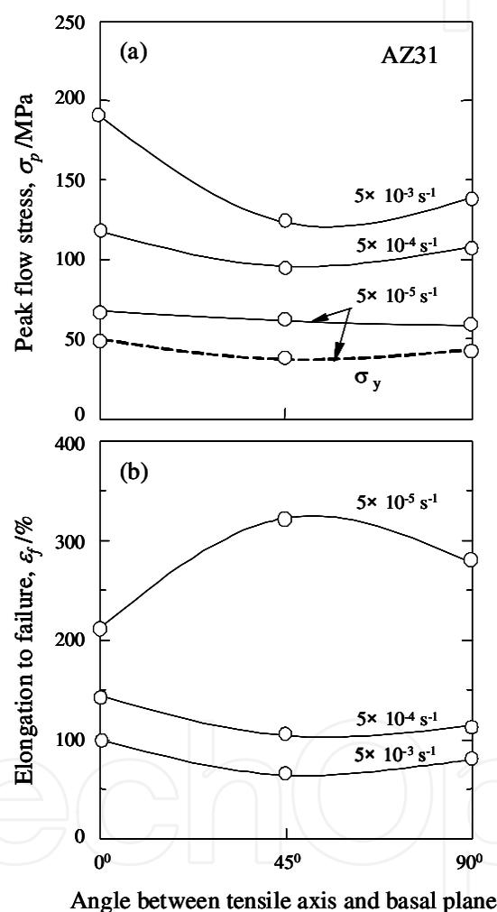
Fig. 23. Changes in (a) peak flow stress  $\sigma_p$  (and  $\sigma_y$ ) and (b) elongation to failure  $\epsilon_f$  with initial textures of MDFed AZ31 alloy tested at 423K and at various strain rates.
