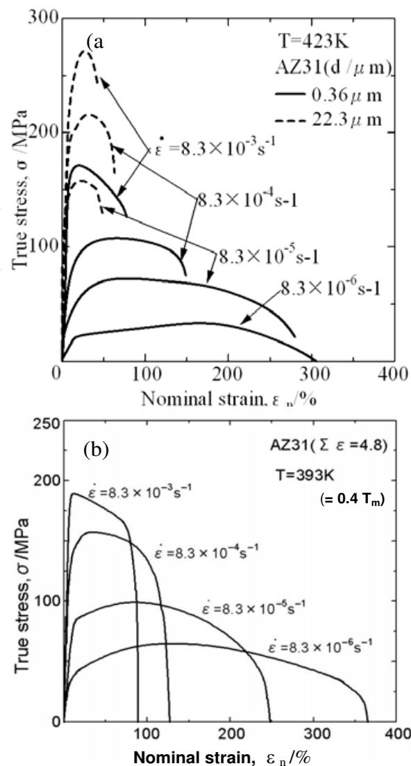
Fig. 18. (a) Effect of grain size on the strain rate dependence of true stress-nominal strain ( $\sigma - \epsilon_n$ ) curves at 423K and (b) strain rate dependence of  $\sigma - \epsilon_n$  curves at 393 K ( $= 0.4 T_m$ ) for Mg alloy AZ31 processed by MDF under dropping temperature conditions.
