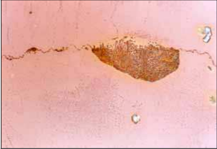
(b) Mg – alloy AZ 63HP, the plate edge, the lamellar precipitate x 500
