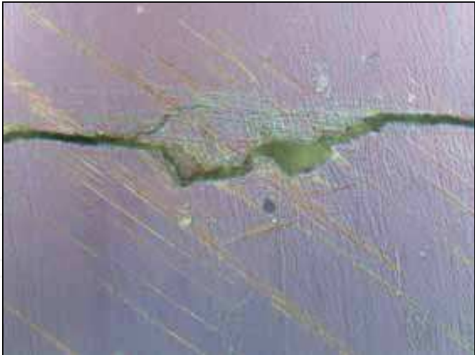
a) transcrystalline fatigue crack growth with the slip bands x 400
