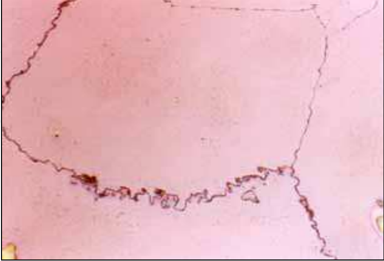
(c) Mg – alloy AZ 63HP, the plate middle, the meandering boundaries x 500
