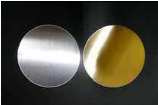
Fig. 4. Photograph of the original Mg alloy sheet (left) and DLC coated Mg alloy sheet (right)
