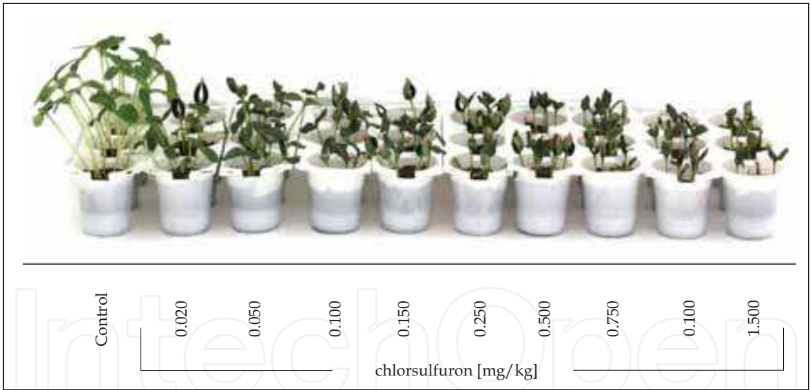
Fig. 5. Te effect of chlorsulfuron on fresh weight reduction of Cucumis sativus (determination of IC 50 )
