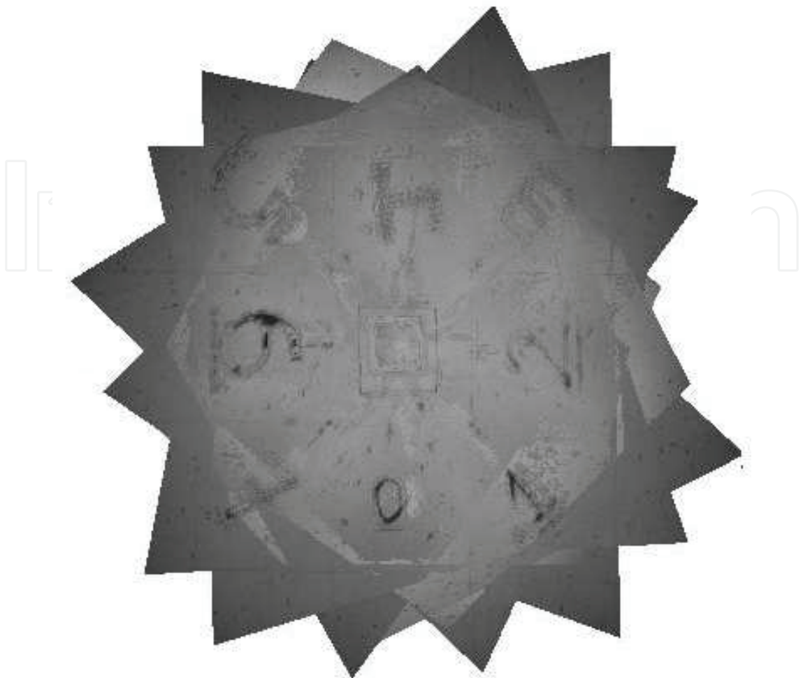
Fig. 11. Single-robot SLAM: generated map of the site
