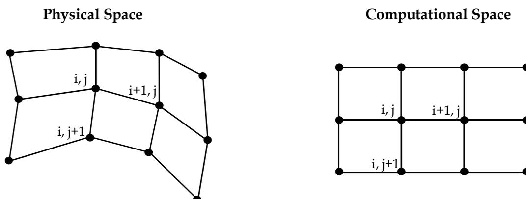
Fig. 1. Mapping associated with a two-dimensional structured grid.
