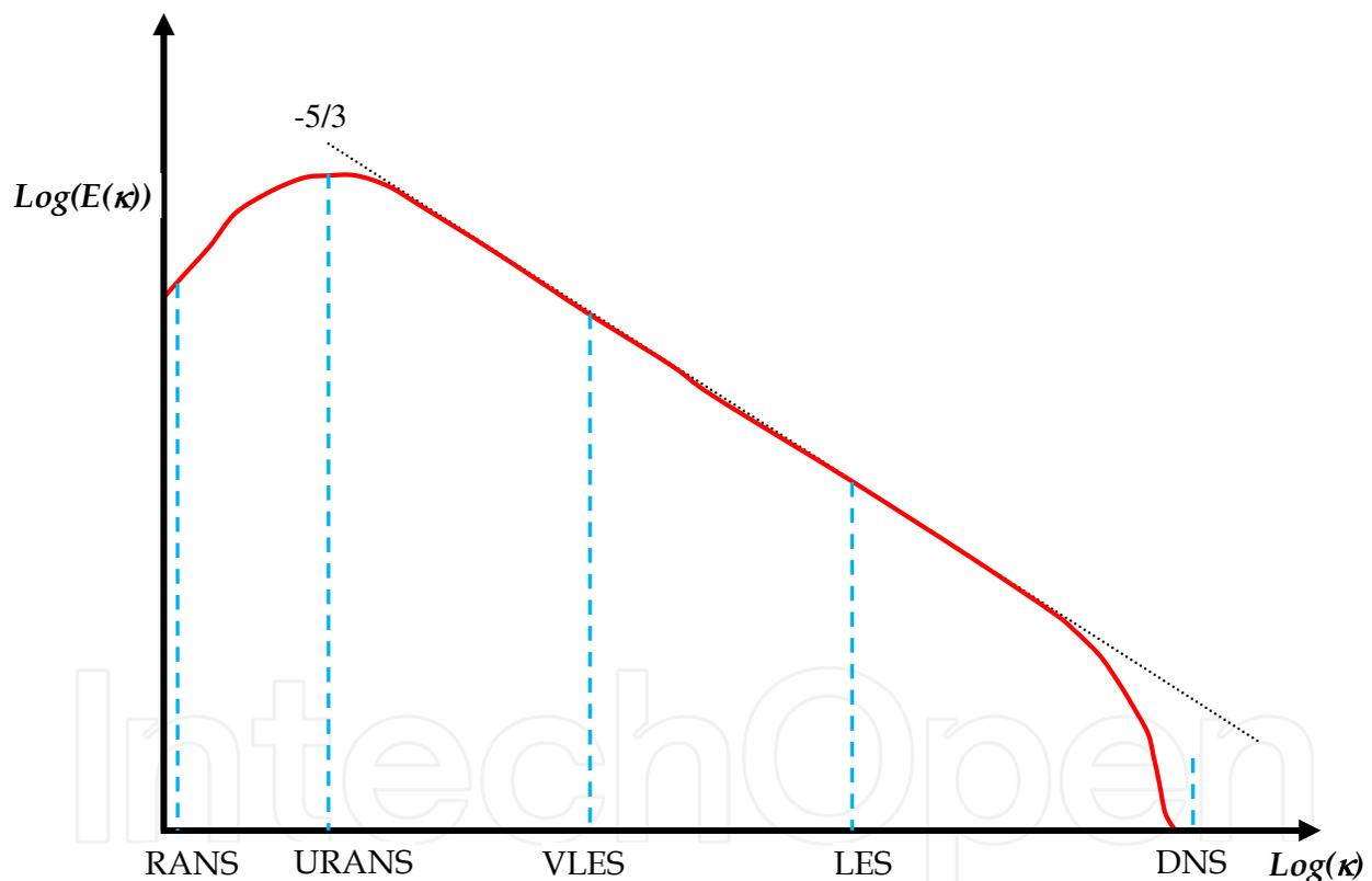
Fig. 3. Schematic view of RANS-DNS resolved energy spectra.
