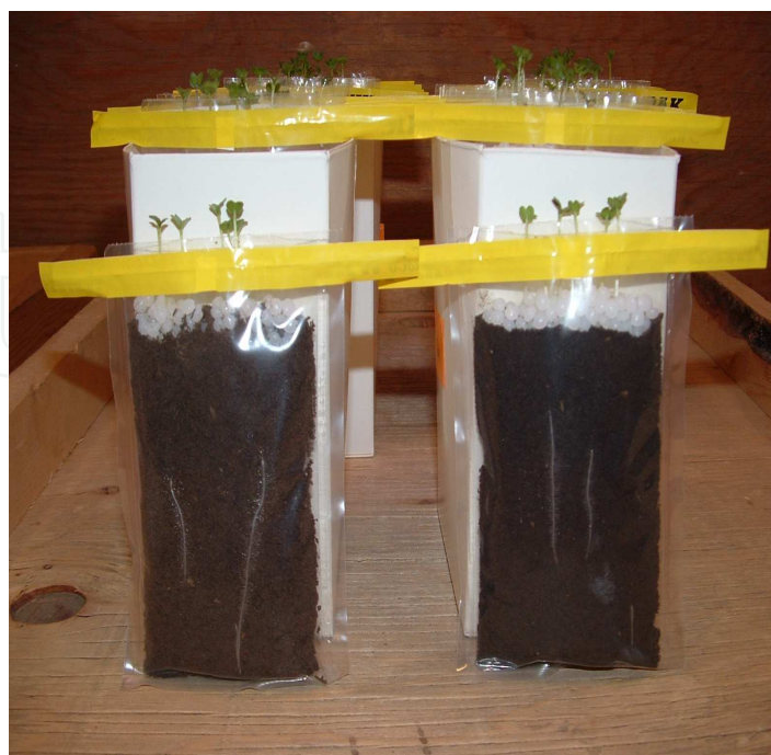
Fig. 1. Mustard root length bioassay performed in Whirl-Pak bags.
