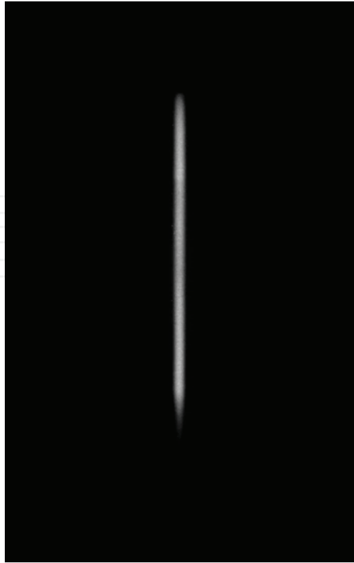
Fig. 2. Black and white silver halide photograph of the emission beam recorded at z = 340 mm. As shown in Duarte et al. (2005) the spatial profile of this single-transverse-mode emission is near-Gaussian and the beam divergence is \sim 1.1 times its diffraction limit (from Duarte et al. (2005)).
