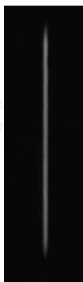
Fig. 9. Black and white silver halide photograph of the near-Gaussian emission beam, from the interferometric emitter (DICOS), recorder under nanosecond pulsed excitation at \sim 10 kV per pulse. The corresponding excitation current density is \sim 190 A/cm 2 (from Duarte (2008)).
