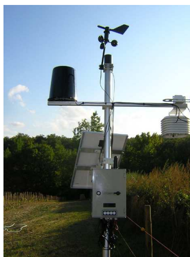
(b) VineSense GPRS Gateway with Weather Sensors
