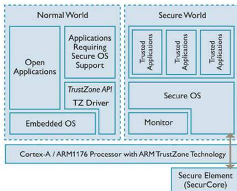
Fig. 2. Trustzone software architecture
