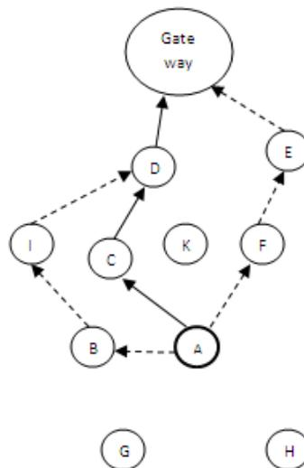
Fig. 3. Trusted node identification in WSN
