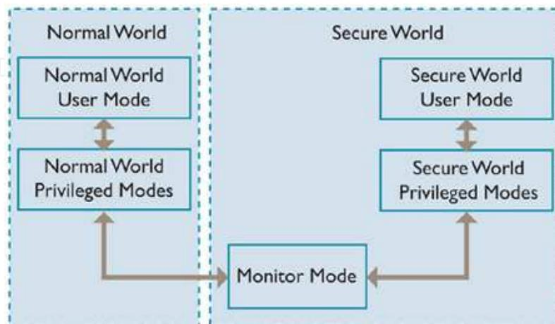
Fig. 1. Trustzone hardware architecture
