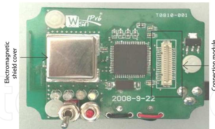
Fig. 14. Main board of the sensor node
