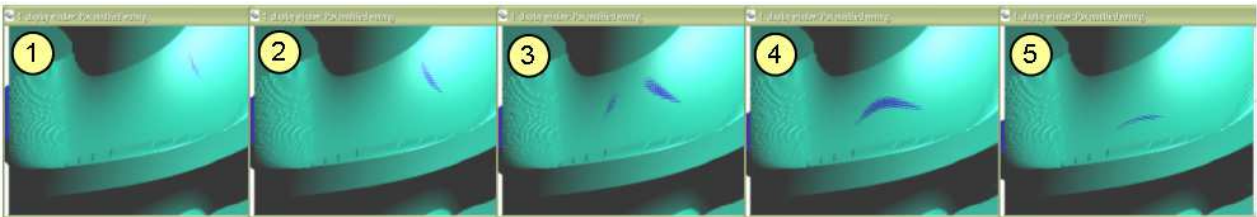
Fig. 31. Contact patterns of the twice modified worm gearing
