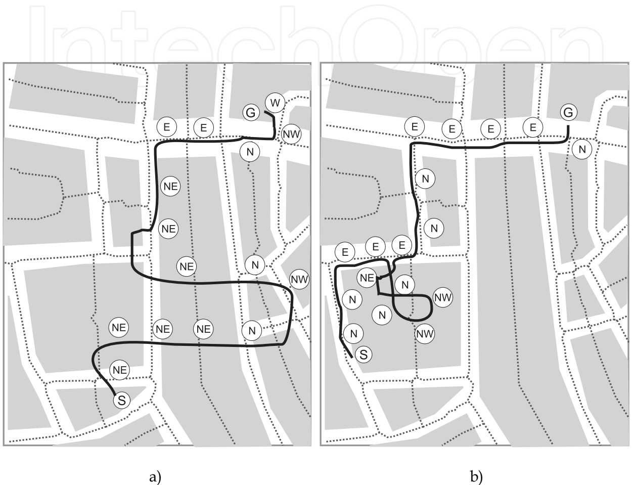
Fig. 6. a) Search mode example: the track of the user's path from start position S to goal position G with the navigational instructions given along the path by TMMS b) Navigation mode example
