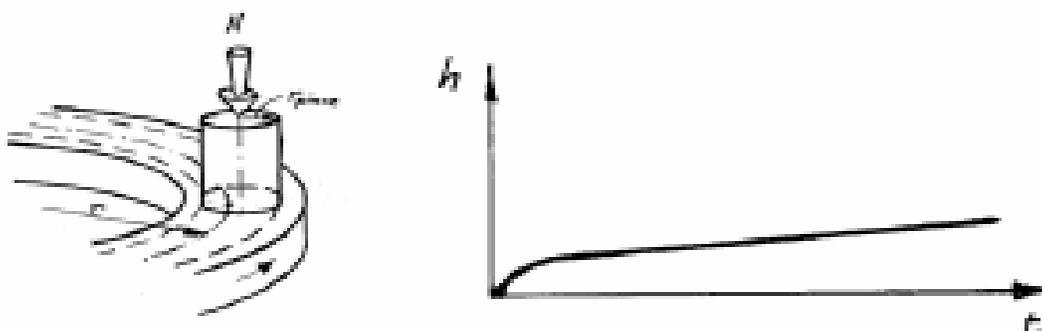
Fig. 1. Pin-on-disc test
