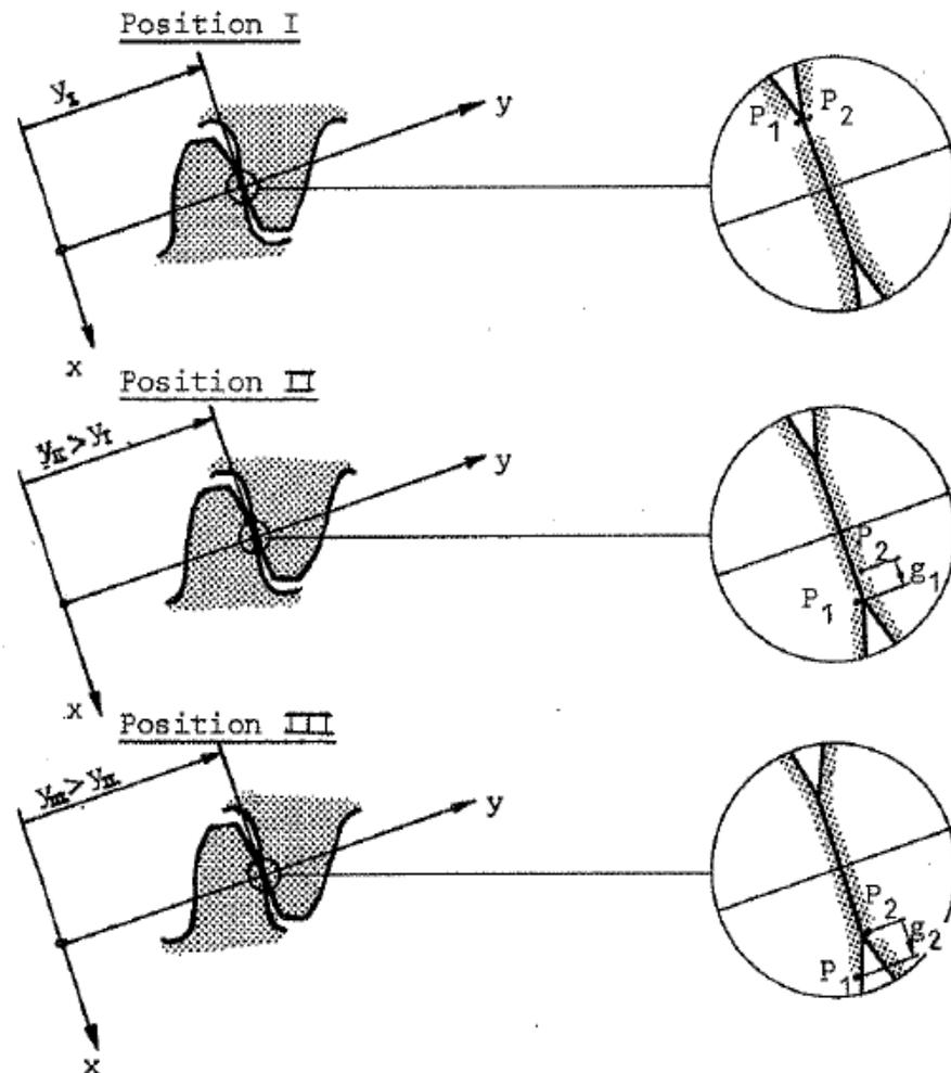
Fig. 9. The distance,  $g_1$ , point  $P_1$  on the pinion flank and the distance,  $g_2$ , point  $P_2$  on the gear flank slide during one mesh; position I corresponds to the moment in time when  $P_1$  and  $P_2$  come into contact with each other, while positions II and III correspond to the moments in time when  $P_1$  and  $P_2$  disengage, respectively. [8]
