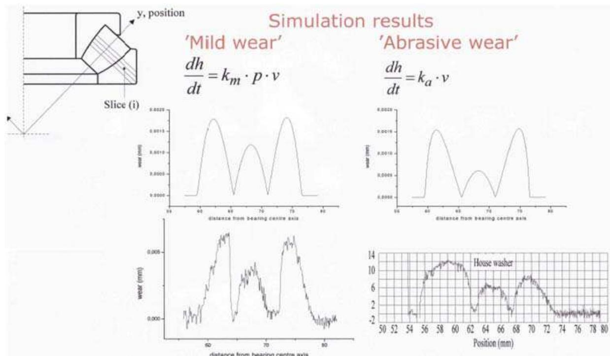
Fig. 3. Abrasive wear compared with mild sliding wear
