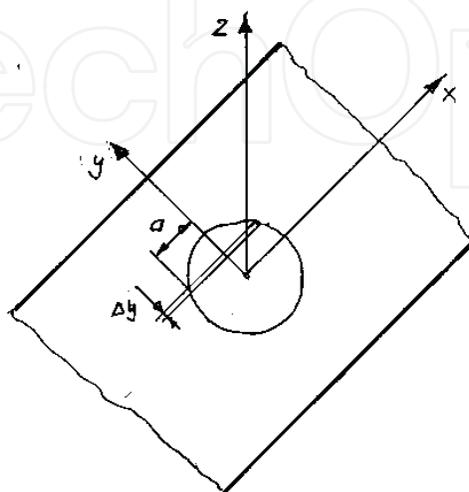
Fig. 13. Contact point and coordinate system, sliced contact
