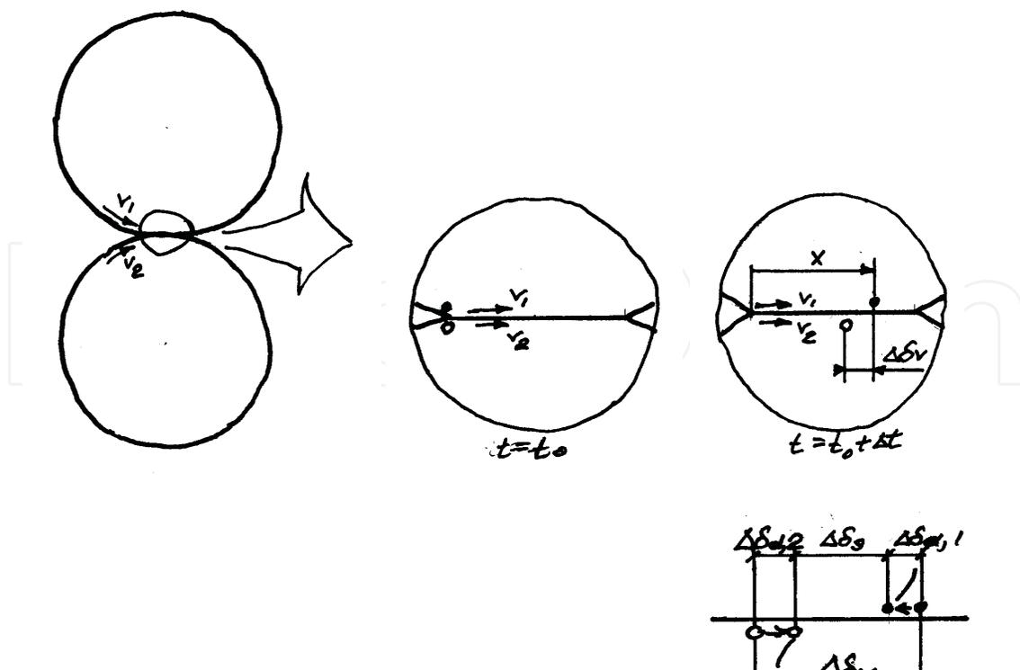
Fig. 5. Two discs: The basic principle for determining the sliding distance in a rolling and sliding contact
