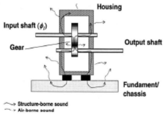
Fig. 18. Noise excitation from a gearbox [22]
