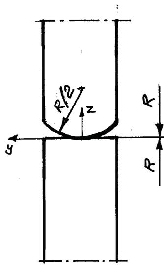
Fig. 12. Interacting modified roller and cylindrical roller
