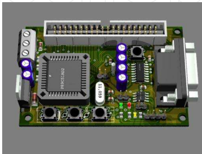
Fig. 3. Example of 3D Model generated from 3DEagle plug-in.
