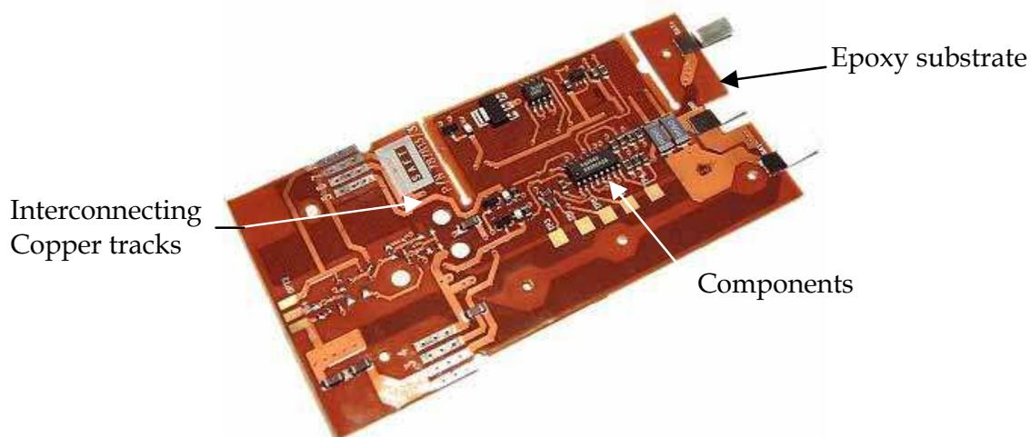
Fig. 1. Populated Printed Circuit Board
