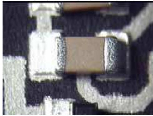
Fig. 23. ECA Printed Correctly
