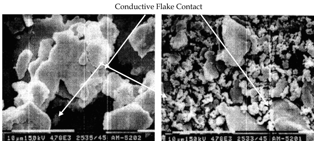
Fig. 6. SEM Micrographs illustrating contact between silver flakes
