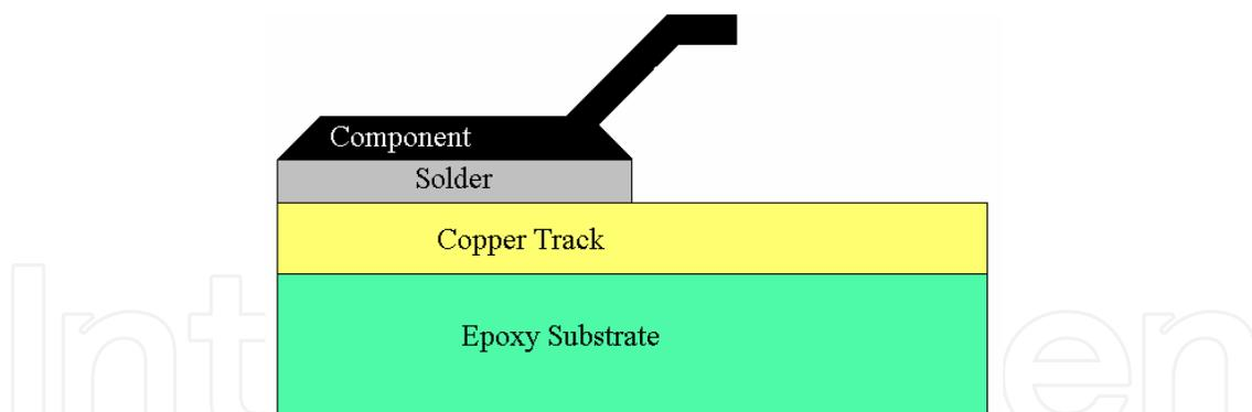
Fig. 3. Surface Mounted Component
