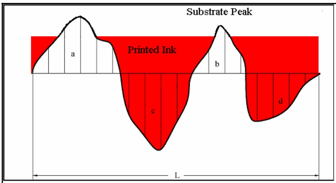
Fig. 8. Example of potential problem of substrate roughness
