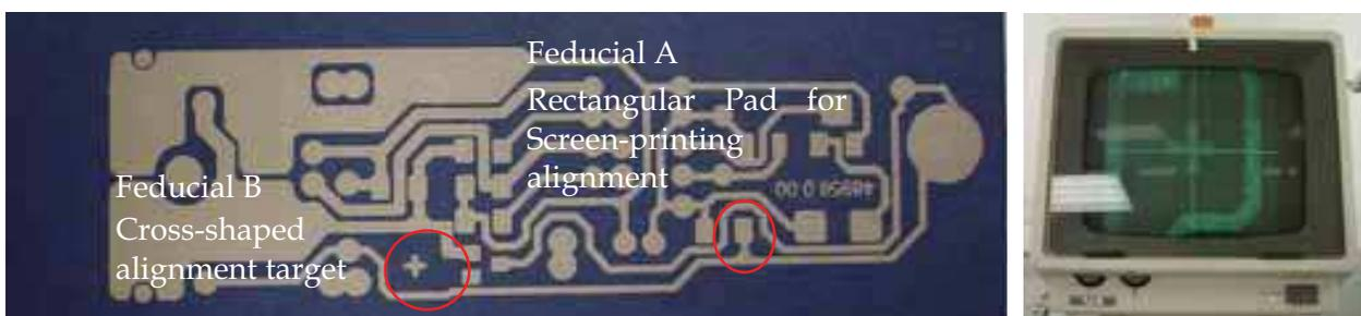
Fig. 18. Feducial used for Vision Alignment
