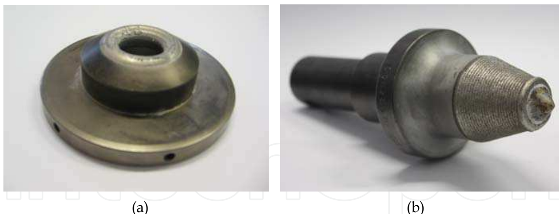
Fig. 11. a) Restored mold component; b) Restored component of the crushing machine
