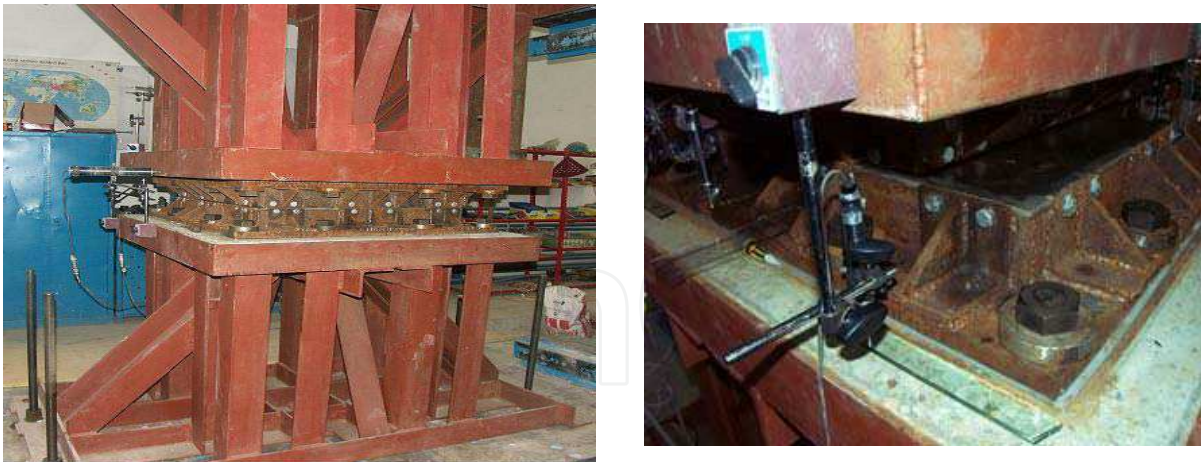
Fig. 2.9. SERB - SITON LP 800 x 800 capsulated isolation device with sliding on plane surfaces
