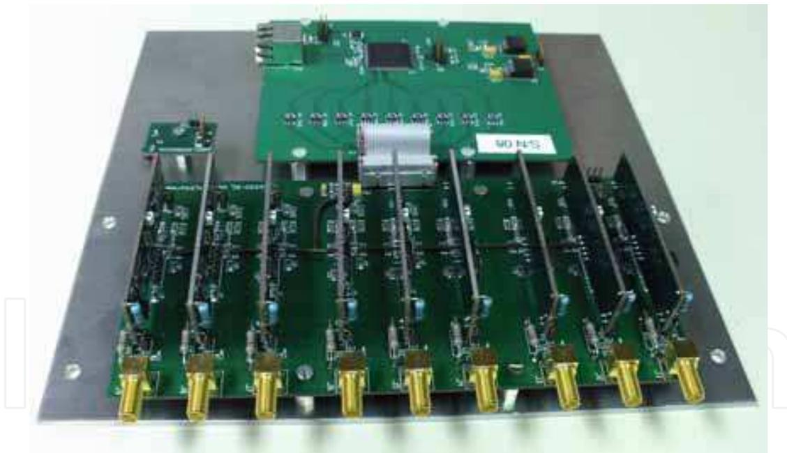
Fig. 12. Electronics for one detector module (Front: Single channel boards on the carrier board; Back: Digitizing board; Small circuit left of digitizing board: 1-wire temperature sensor).
