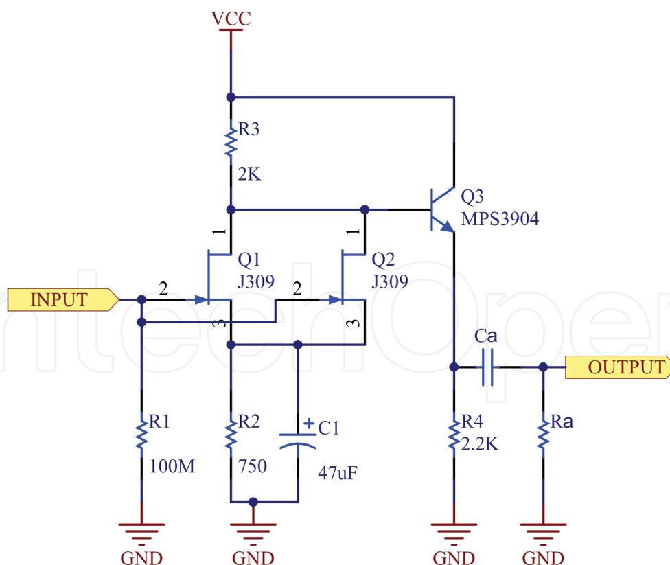
Fig. 13. First stage of the preamplifier in version 1.
