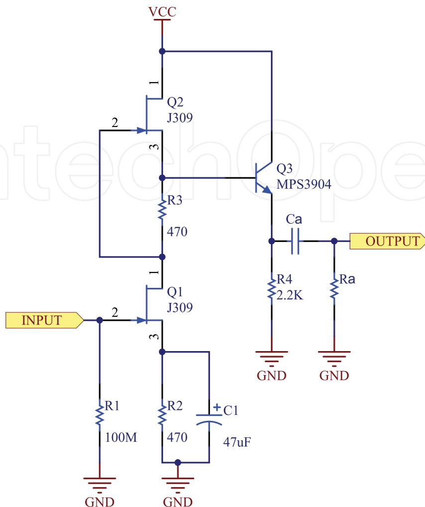
Fig. 14. Part of the microphone amplifier schematics used in the second version of the PICASSO preamplifier.
