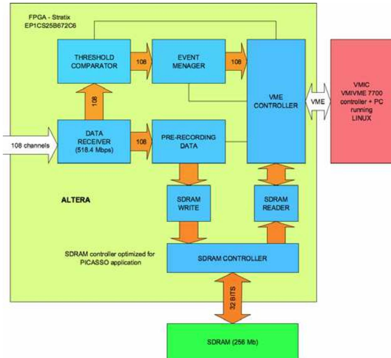
Fig. 18. Functional block-diagram of a collector board.
