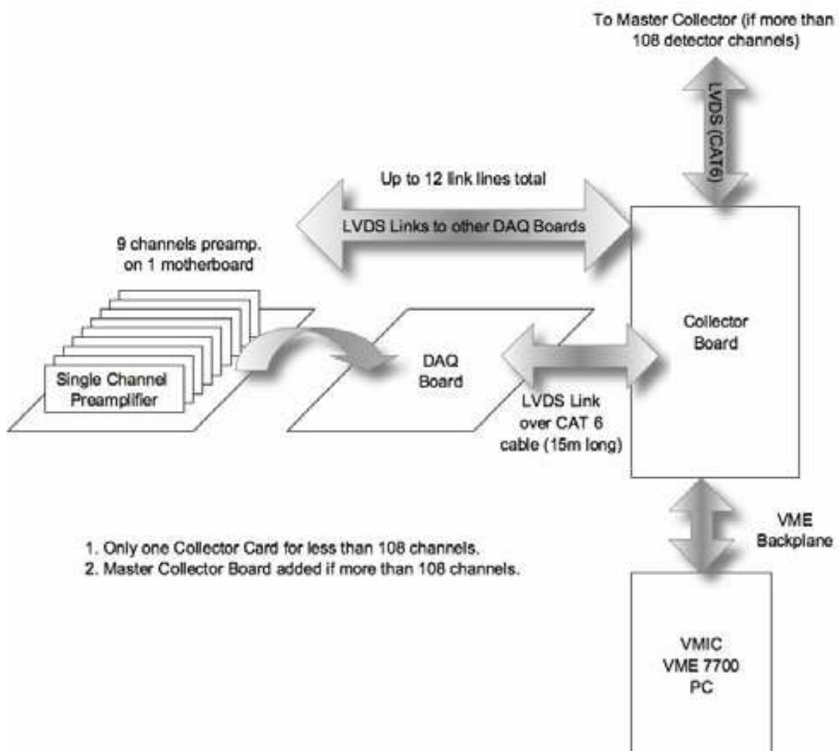
Fig. 9. Functional block-diagram of signal and data flow.
