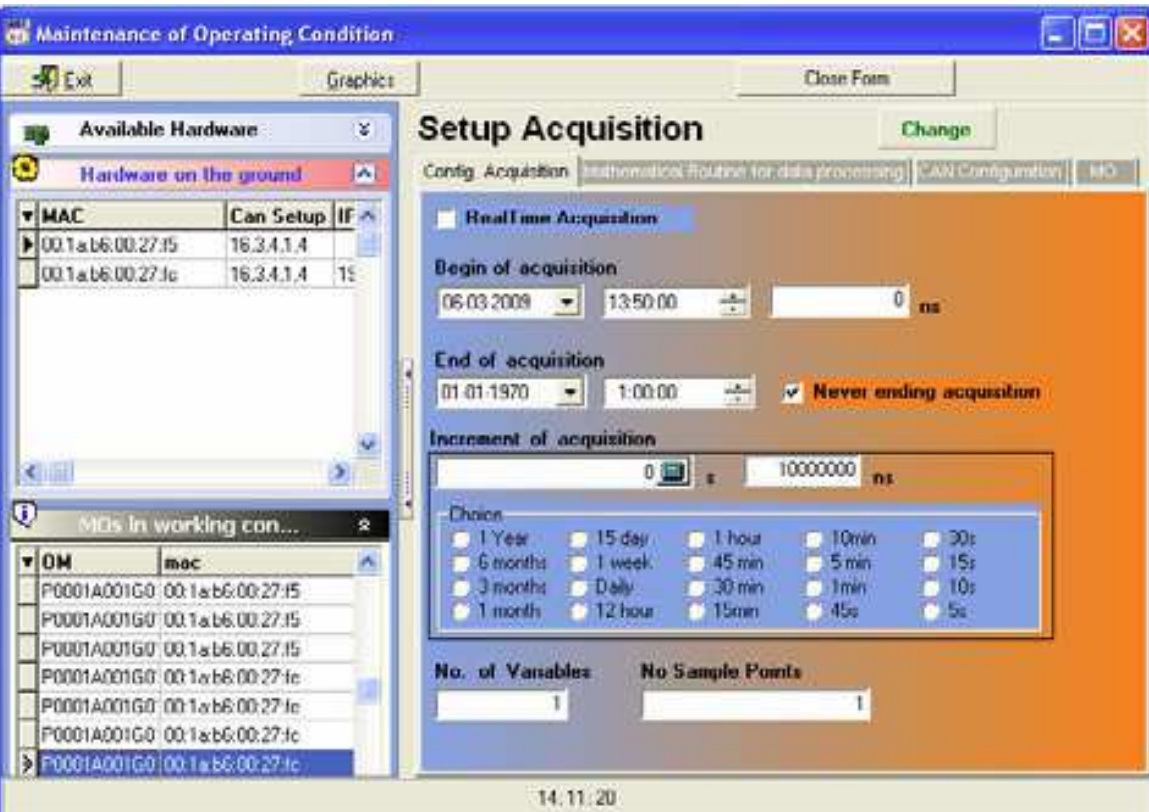
Fig. 8. Programming the acquisition temporization for each low cost I/O board in the SMIT's on-condition module (Fonseca; 2010).
