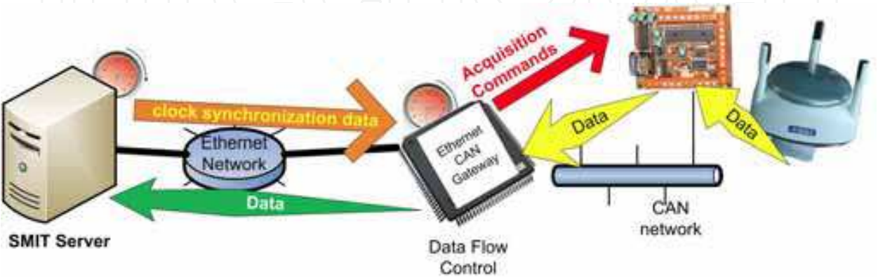
Fig. 2. Information flow between different SMIT's components (Fonseca; 2010).
