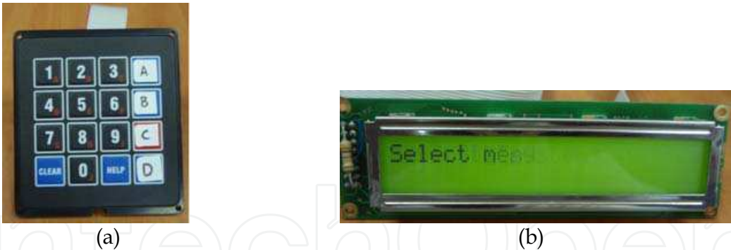
Fig. 6. a) 4x4 matrix keypad b) 24x2 alphanumeric LCD panel
