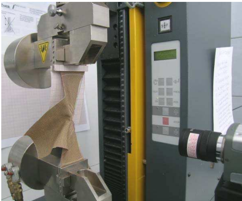
Fig. 4. The way of sample mounting in the tensile machine jaws for the tearing zone registration Source: own
