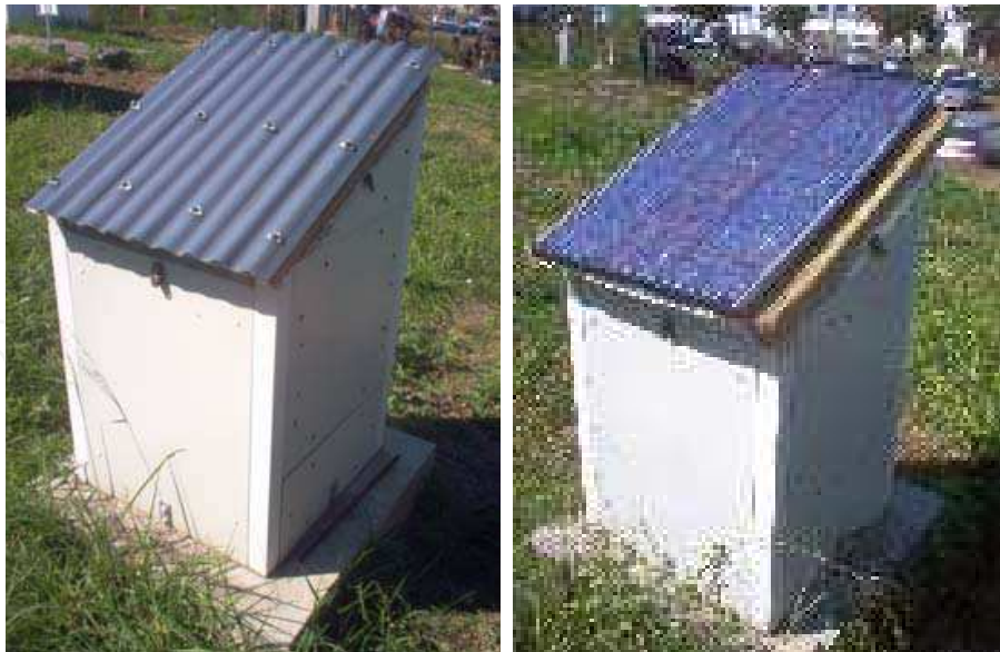
Fig. 9. Photography of Isotest cell without and with PV panel.
