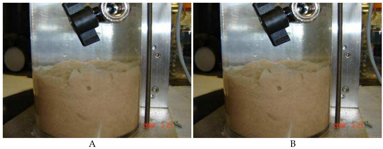
Fig. 15. Coated sand with xanthan and guar gum did not exhibit erosion at speeds of 3.7 m/s (A) or 11m/s (B).
