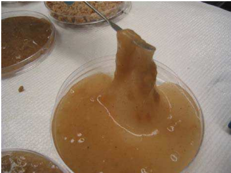
Fig. 11. Adhesive product of sand coated with guar gum cross-linked by borax.
