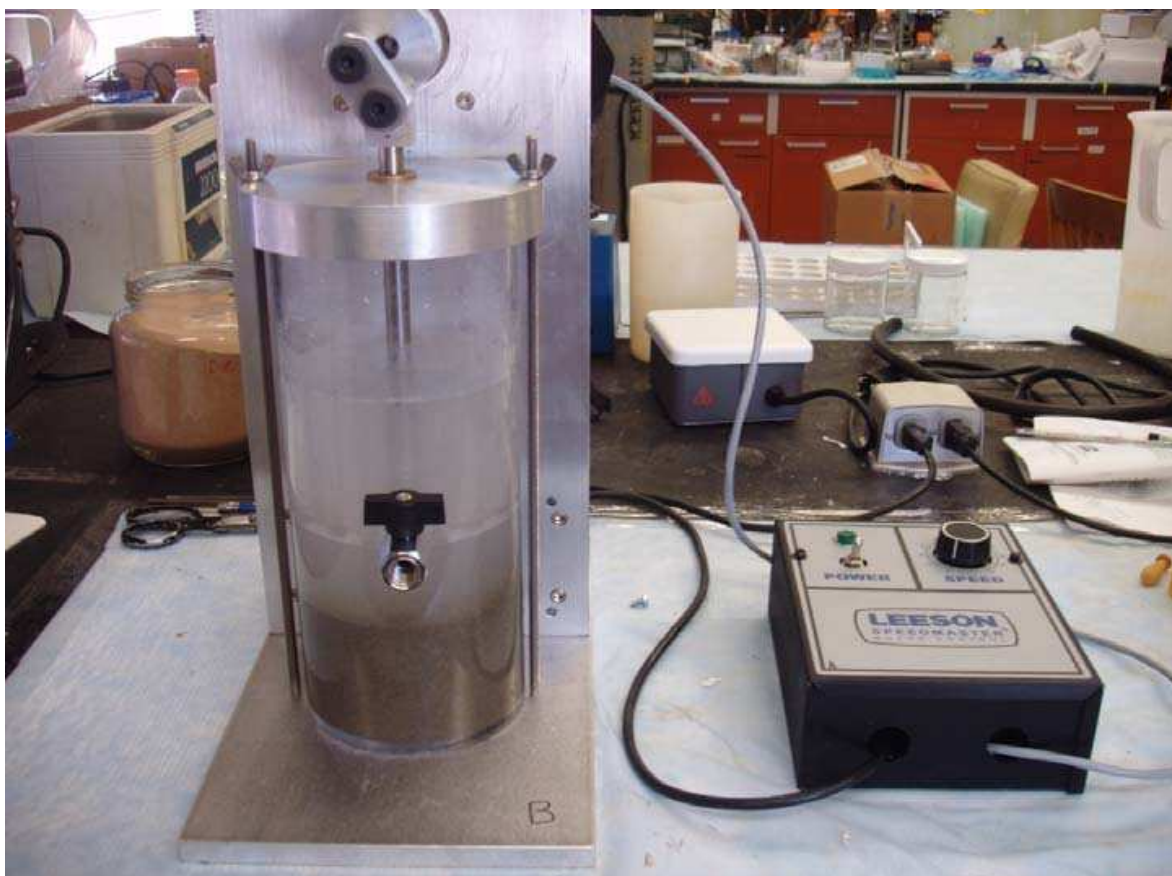
Fig. 1. Shaker for simulating erosion.
