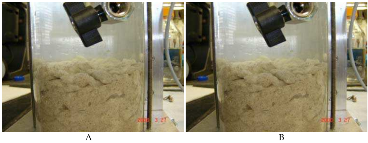
Fig. 16. Sand and organoclay (PM-199) mixed with the biopolymers xanthan and guar gum did not show erosion at speeds of 3.7m/s (A) or 11m/s (B).
