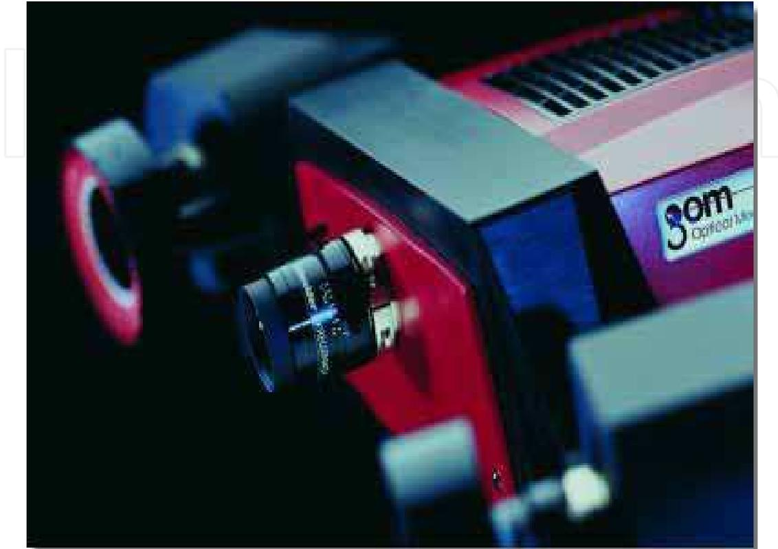
Fig. 6. Scanning digitiser camera
