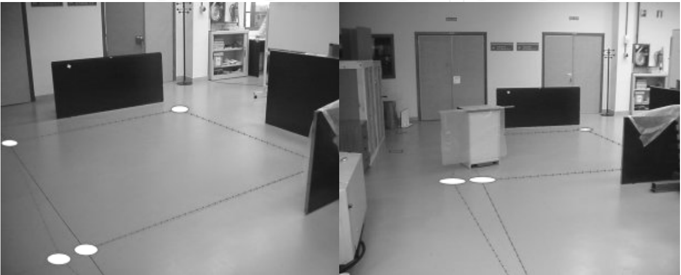
Figure 12. Lab workspace setup: an area of 130 square meters, and a point-to-point mission of a length of 55.6 meters with 12 checkpoints
