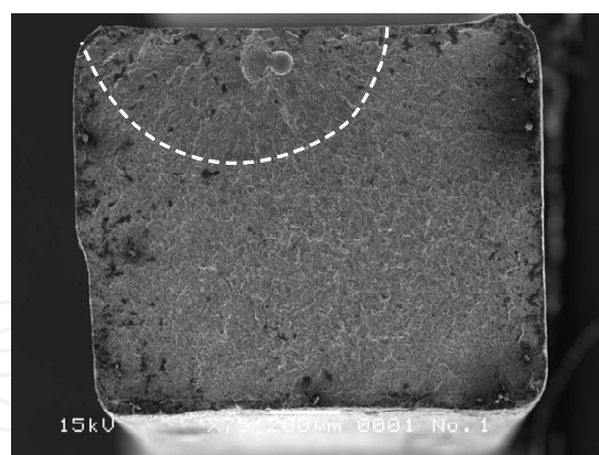
Fig. 18. SEM photograph of fracture surface for cast SMA in alternating-plane bending fatigue
