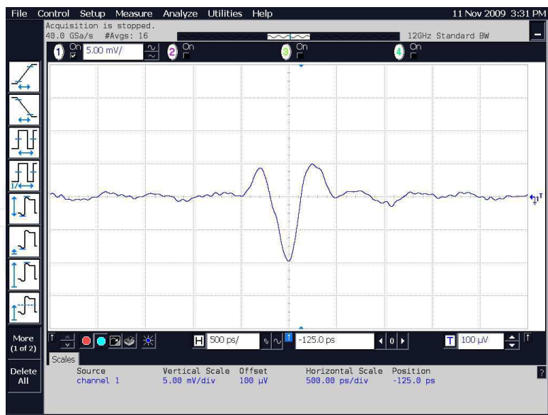
Fig. 7. The measured Gaussian doublet at the output of the passive UMZI system
