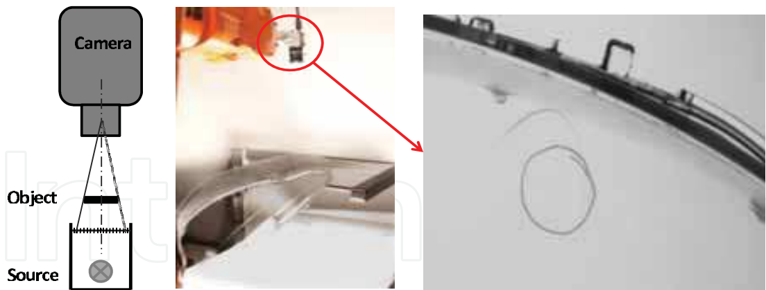
Fig. 9. Diffuse back-light. From left to right: principle of lighting; robotic platform with back-light illumination; the image acquisition.
