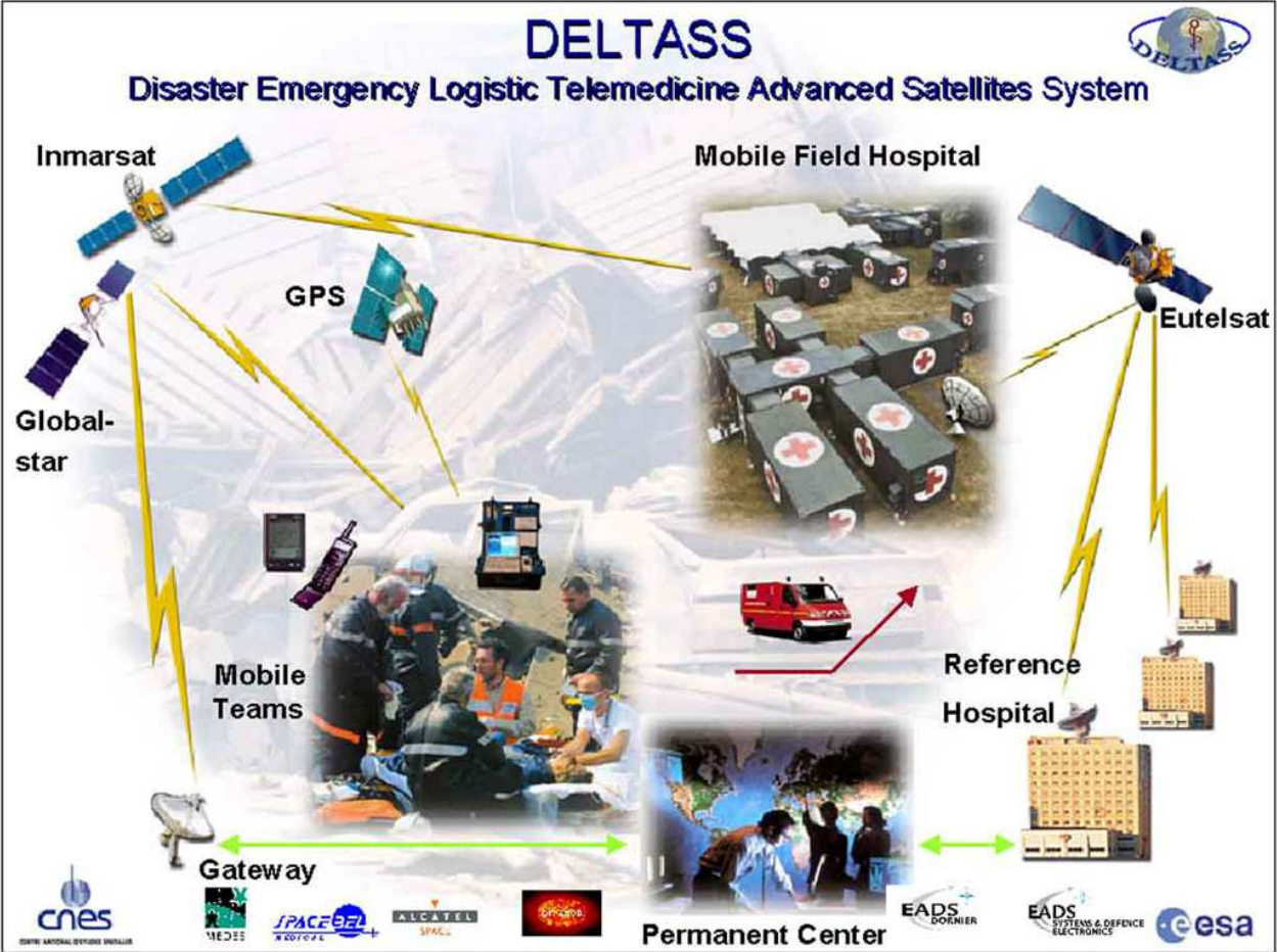
Fig. 2. DELTASS System Architecture: Mobile Teams, Permanent Centre (PC), Mobile Field Hospital (MFH) and Reference Hospital (RH) are interconnected via several satellite systems with different bandwidths. Additionally, terrestrial communication channels support the data exchange between the PC and the RH.
