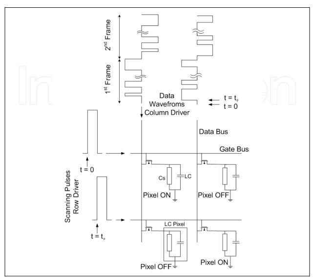
Fig. 7. Configuration of the active matrix addressing method.
