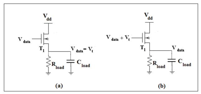
Fig. 17. (a) Typical source follower topology, (b) Source Follower topology with threshold voltage compensation.
