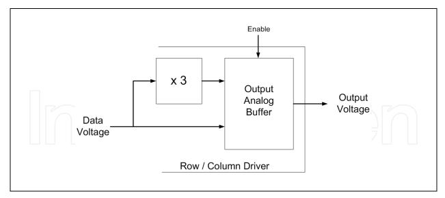
Fig. 19. Row/Column driver architecture with the use of the static source follower.
