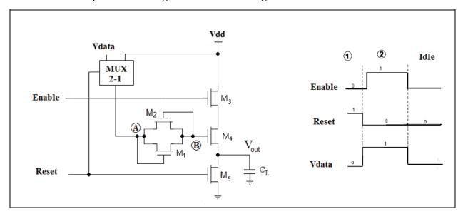
Fig. 20. Dynamic source follower topology with its timing diagram.
