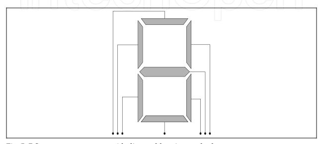
Fig. 5. 7-Segment arrangement with direct addressing method.
