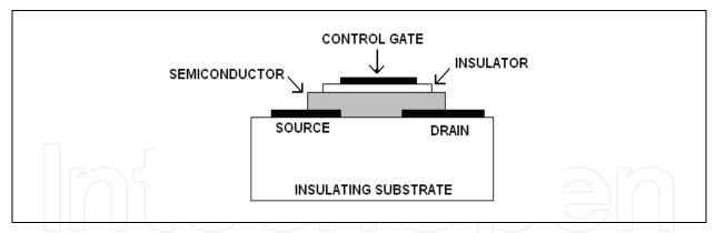
Fig. 1. Schematic diagram of Weimer's staggered CdS TFT structure.
