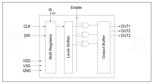
Fig. 15. Basic architecture of a row driver.
