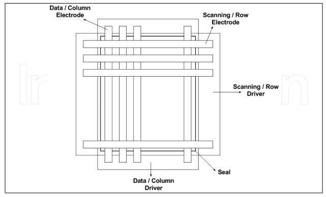
Fig. 6. Configuration of the passive matrix addressing method.
