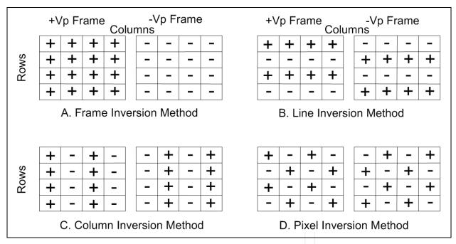
Fig. 13. Typical AMLCD polarity inversion methods.
