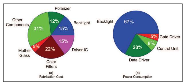
Fig. 9. (a) Fabrication cost contribution of each component. (b) Power consumption contribution of each electronic module.
