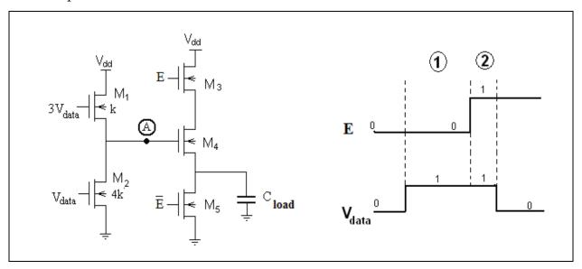
Fig. 18. Static source follower topology with its timing diagram.
