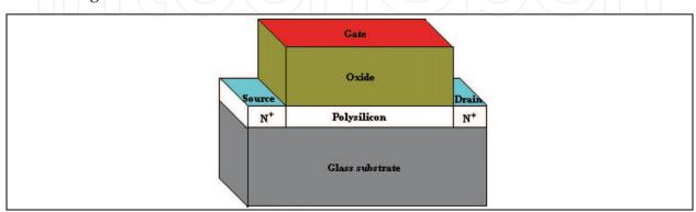
Fig. 3. Poly-Si top-gated TFT structure.
