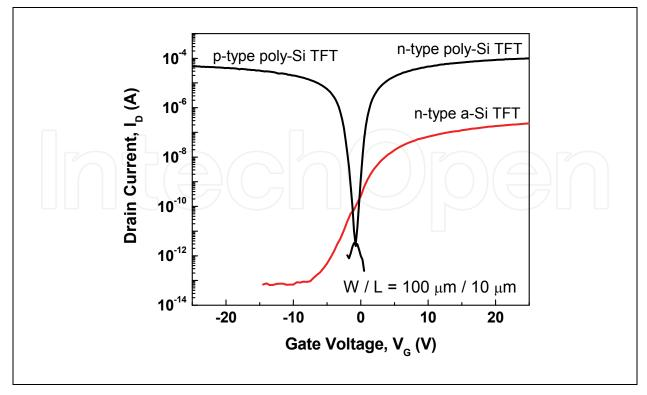
Fig. 4. Transfer characteristics of polysilicon and amorphous TFTs.
