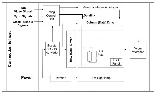
Fig. 8. Block diagram of an AMLCD architecture.
