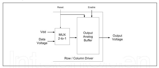
Fig. 21. Row / Column driver architecture with the use of the dynamic source follower.
