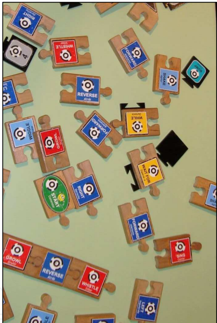
Fig. 18. This tangible interface consists of wooden blocks shaped like jigsaw puzzle pieces (Horn2009)
