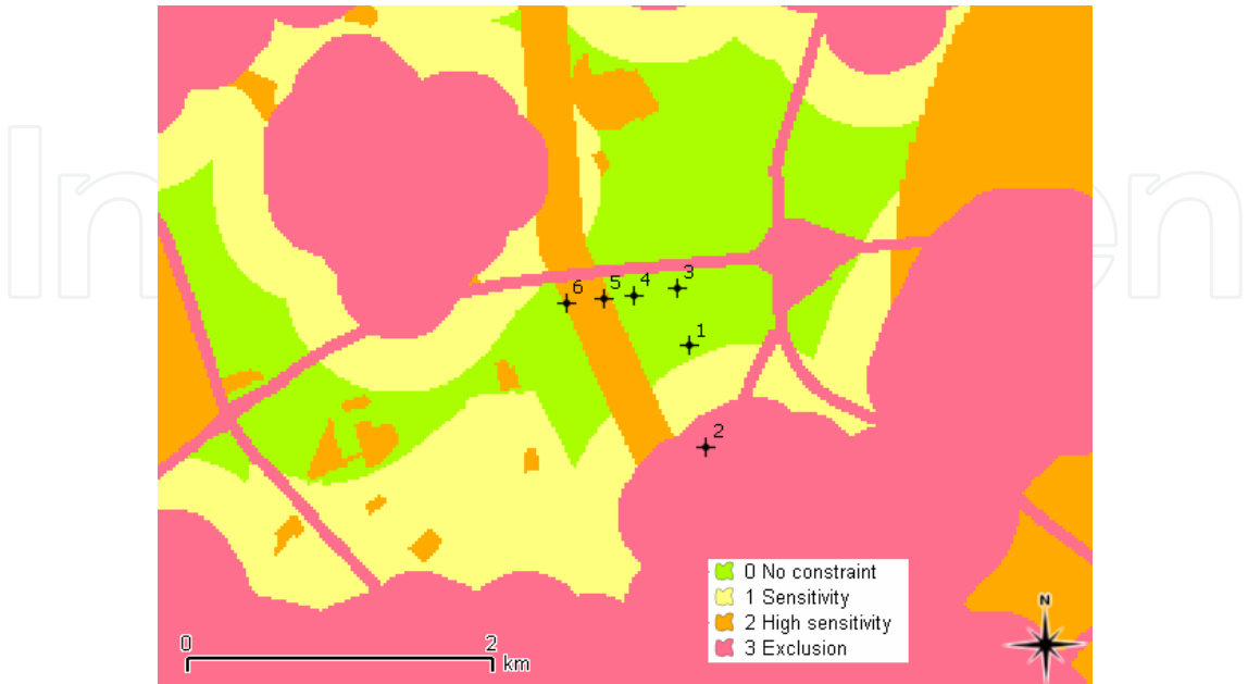
Fig. 10. Overlay of the location of a wind farm project and the composite constraints map.
