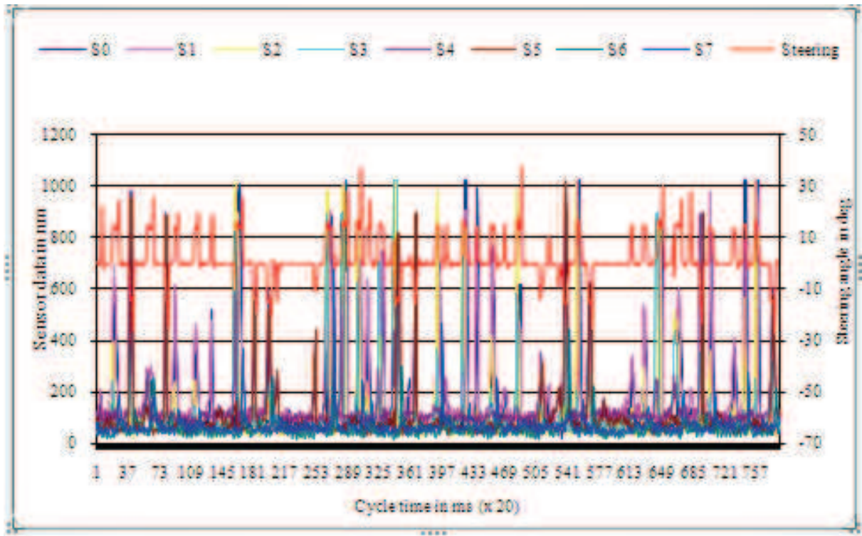
Fig. 6. Graph showing the cycle time plotted against the sensor readings in mm sensors S0 to S7 and steering angle. The final path travel is computed from the total control cycle time and the speed of the robot, which kept as same value in all experiments. The near optimal path is achieved by behaviour rule selection using the 3- alpha fuzzy intervals when more than one behaviour rules of the same kind is present in the environment during navigation. A small portion (period around 280 x 20 ms, 300 x 20 ms and 345 x 20 ms) of the output results of Figure 6 are enlarged and shown in Figure 7.
