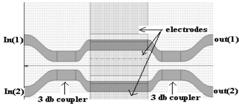
Fig. 3. 2 x 2 MZI switch layout
