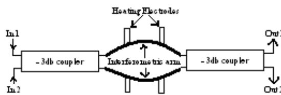
Fig. 2. Basic 2x2 MZI switch structure, ref. [10]
