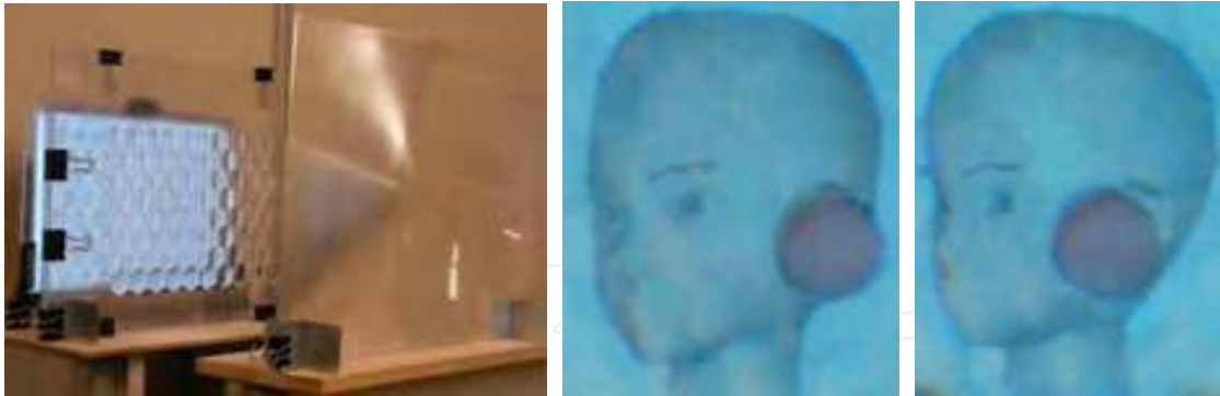
Fig. 17. Prototype of coarse integral volumetric display using DFD for distorted image plane and hexagon component lenses (left) and the images observed from two different viewpoints with the prototype system (middle and right).
