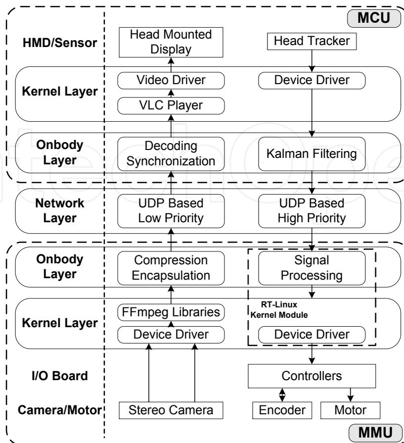
Fig. 3. Flowchart of the stereo vision software architecture.
