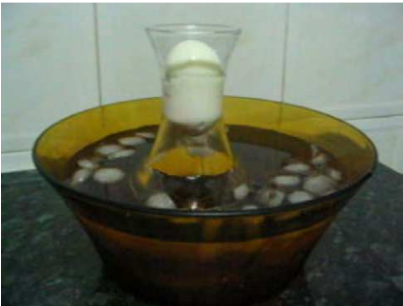
Fig. 2. Egg moving downwards by pressure difference
